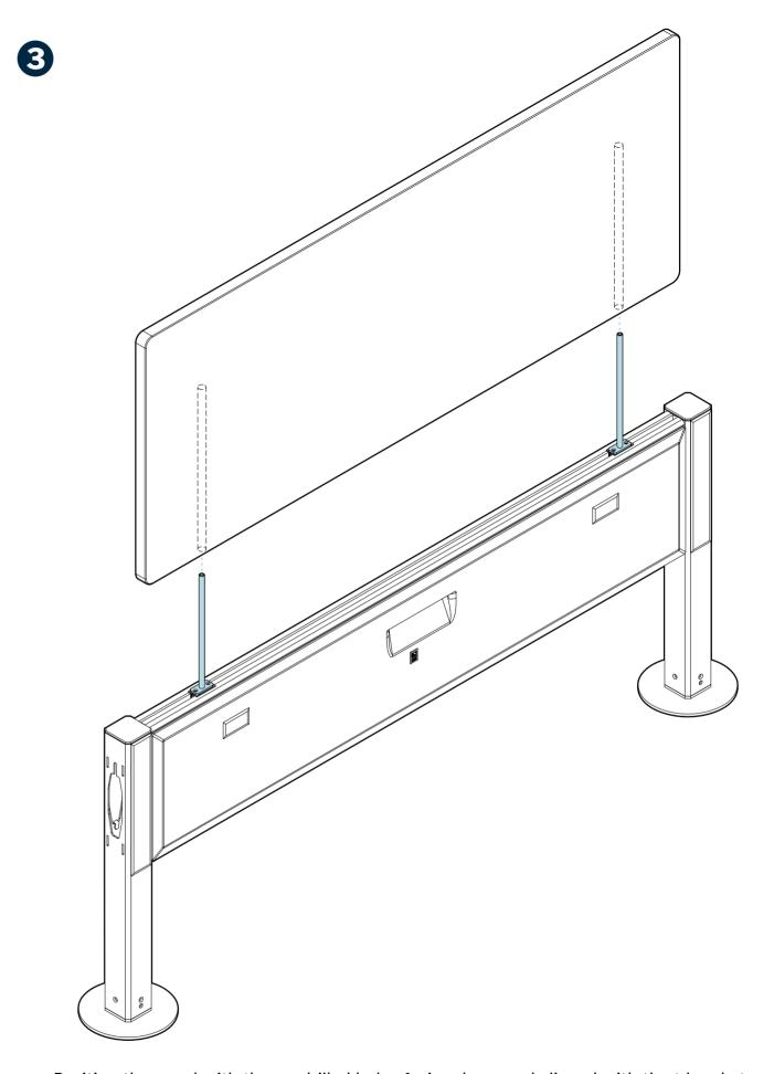
Position the panel with the predrilled holes facing down and aligned with the t-brackets, then lower the panel onto the t-brackets.
